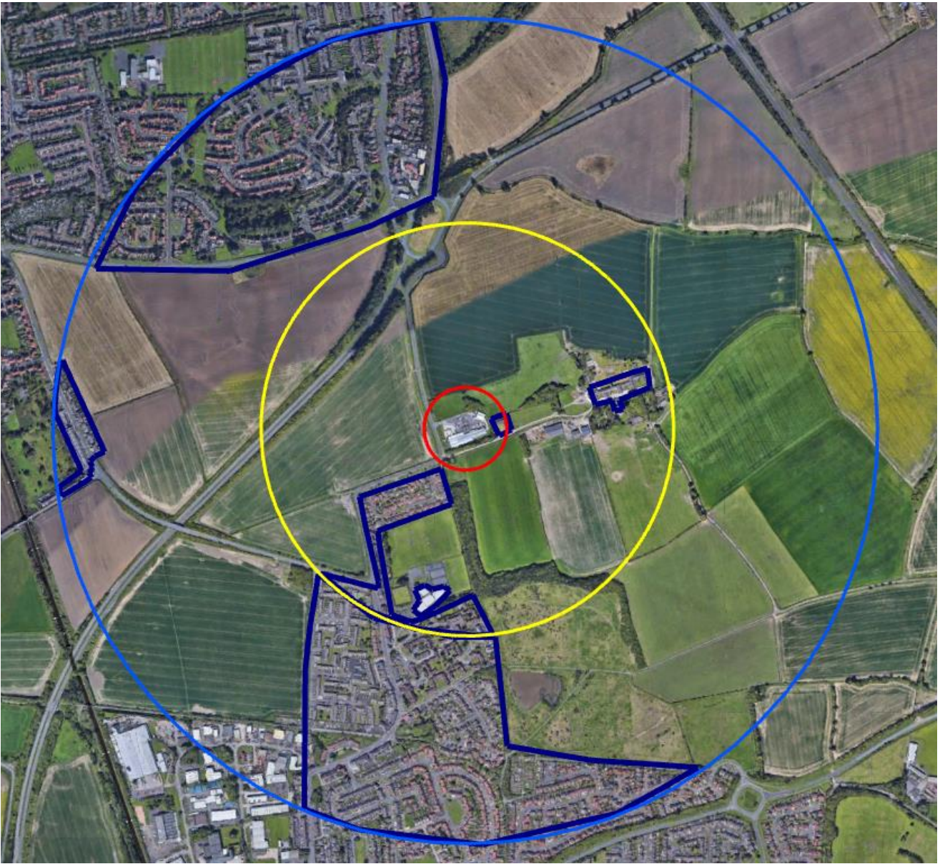
Figure 1 Site area map with zones of sensitive receptors, 100m(RED), 500m(YELLOW), 1000m(BLUE) & Receptors (NAVY).
