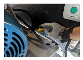
The spanner (provided) is used to unscrew and clean the blue filter and clean under the tap or with a hose pipe. Ensure that the seal is inserted and that the filter is tightened so as not to leak water
