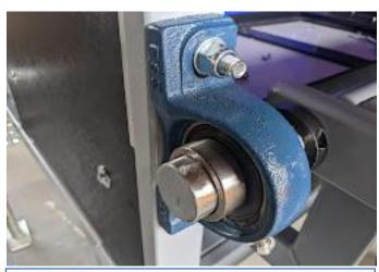
Always lubricate via the grease nipples
