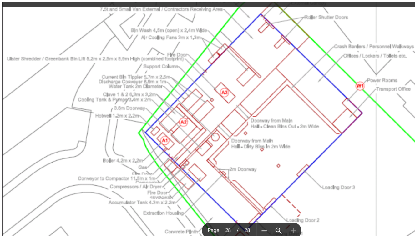
Figure 2: Locations of Equipment to be surrendered (Autoclave, Boiler and Binwash)
