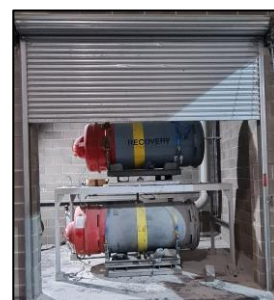
Photographs of the Cooling Unit Treatment Plant Photograph (5): The sealed shredder unit. Photograph (6): Liquefied CFC / Pentane output.
