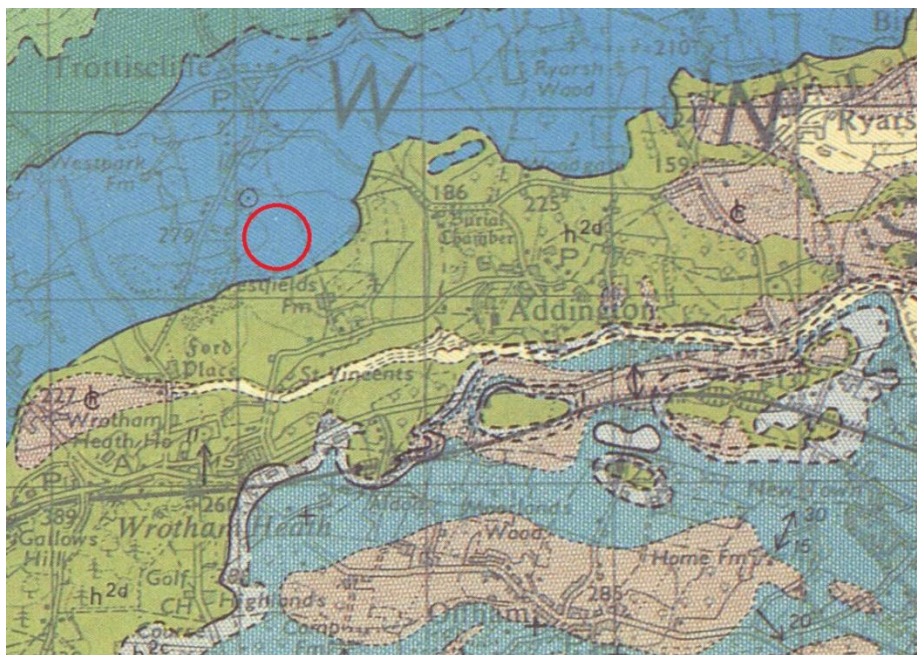
Image 1: Local Geology with Gault Clay strata in dark blue and Folkestone Bed strata in light green (Not to Scale)
