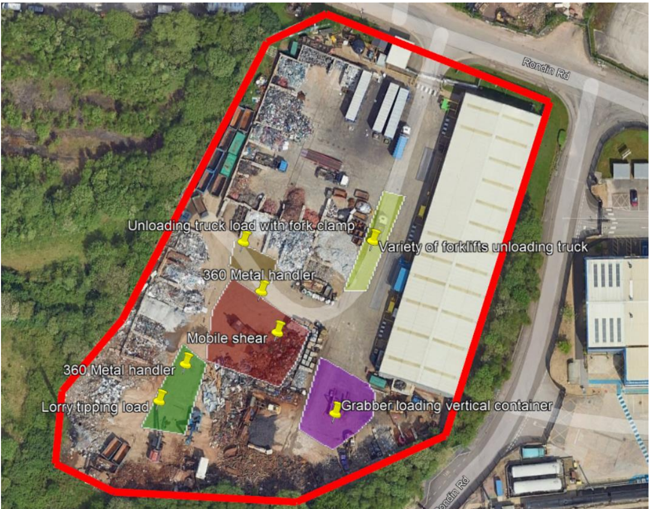
Figure 4-2 Locations of noise sources on site
