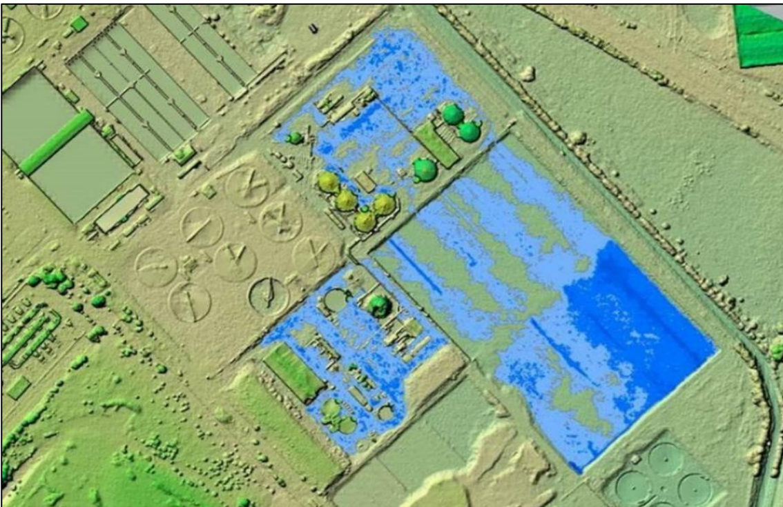
Figure 23. Scenario 3: Model output of spills from existing tanks in Area A and B (110% of each volume) within the permit area at Knostrop.
