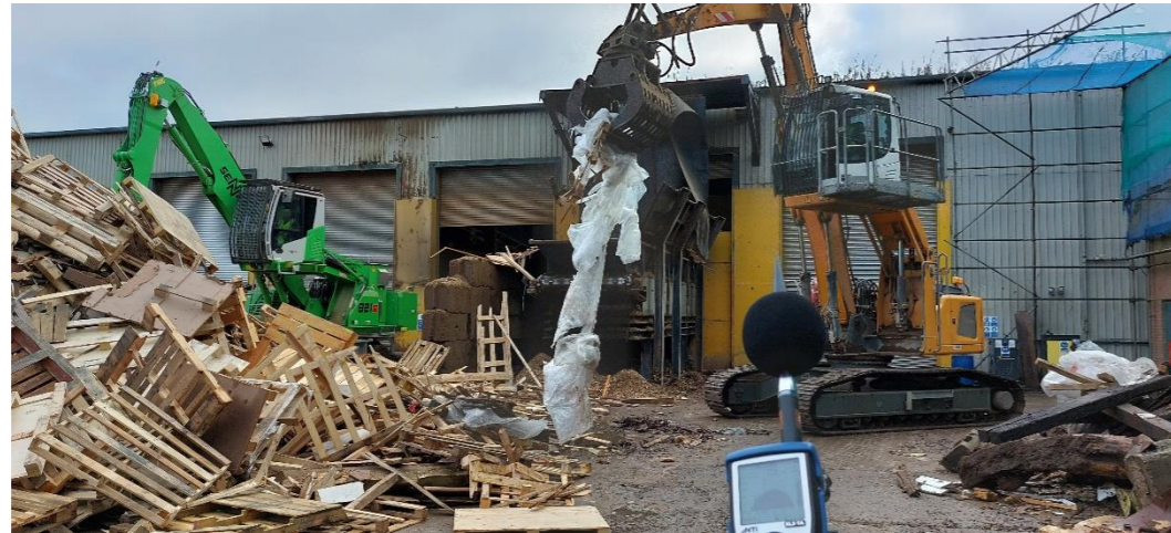
Figure 8: Measurement of the shredder and feeding grabbers
