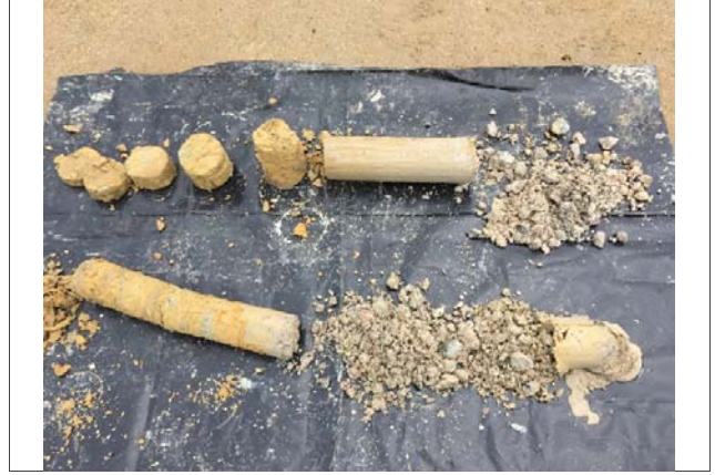
14: Typical Geology in the Central Slab Area
