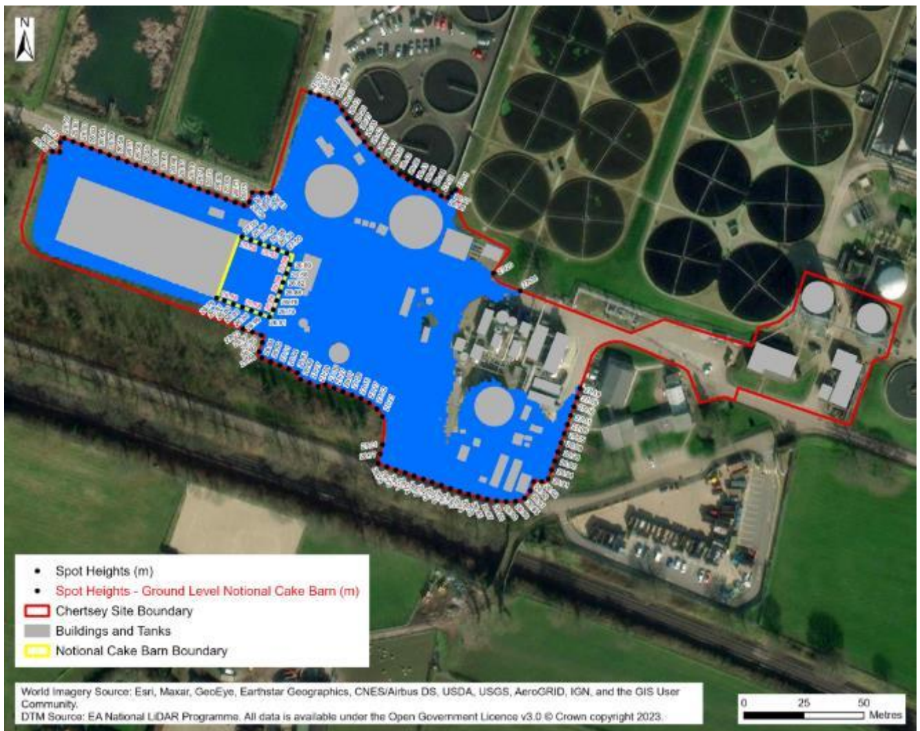
Figure 9- Spot Levels along Containment Boundary
