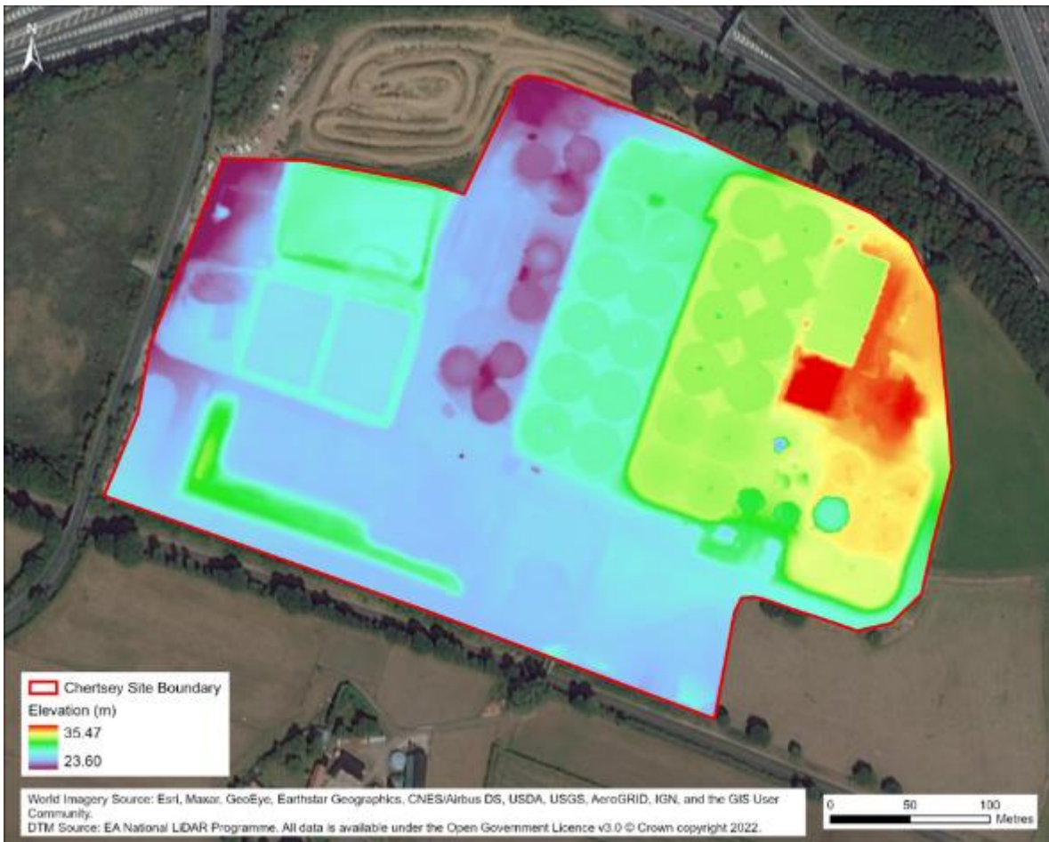
Figure 6- Digital Terrain Model of Chertsey Sewage Treatment Works
