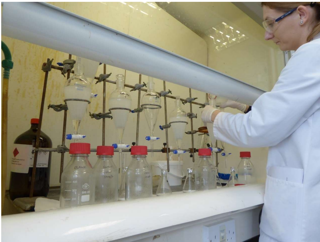
Figure 1. Solvent liquid separation of phases to clean and remove water from samples
