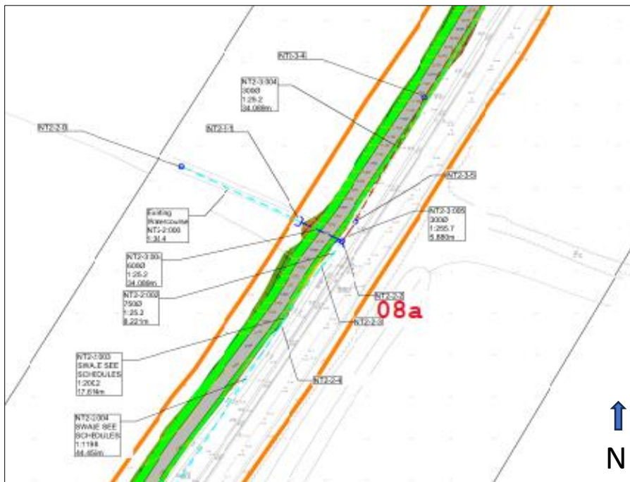
Figure 10 - Outlet O8a Discharge Location
