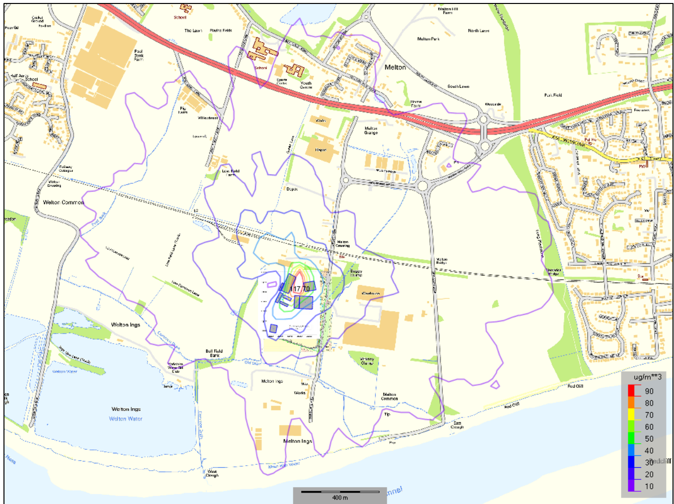
Figure 6-7. Predicted Ground Level Short-Term NO 2 Concentrations (PC, 1-Hour Mean, 99.79 th Percentile) from the Operation of Eco-Power Boilers (2018 Met Data) – Scenario 2
