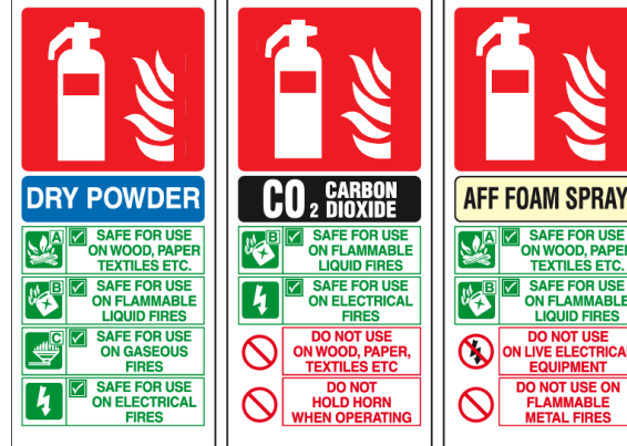
Figure 6: Fire Extinguishers Type and Application
