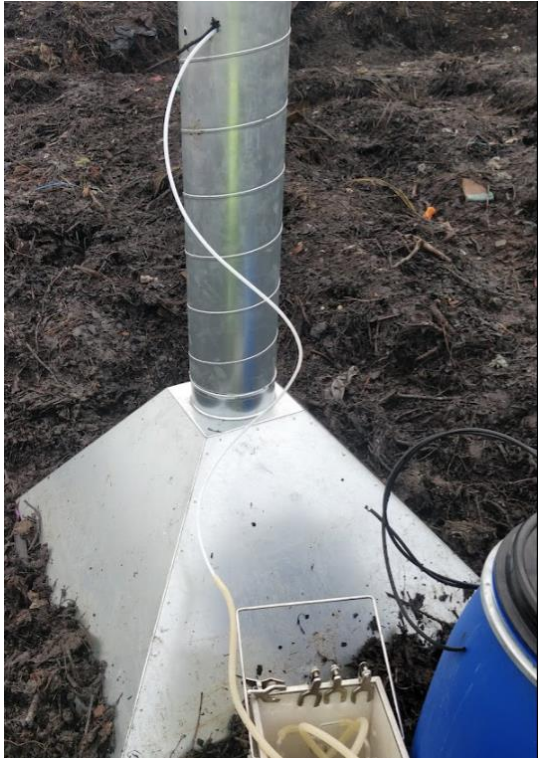
Sampling using a passive sampling hood
