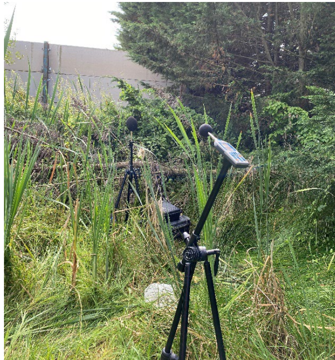
Figure 5. Measurement position setup long-term SLM in background (view facing southeast)
