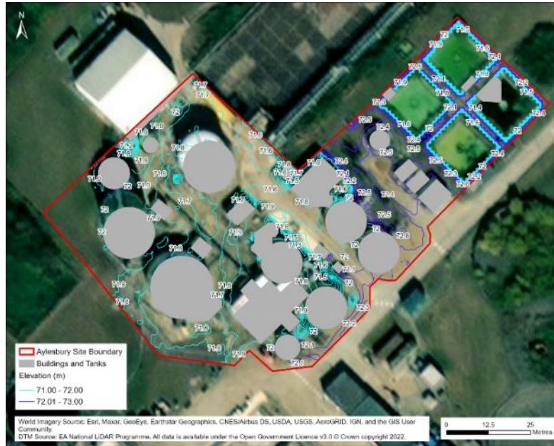
Figure 3-4 Contour lines within containment area 1
