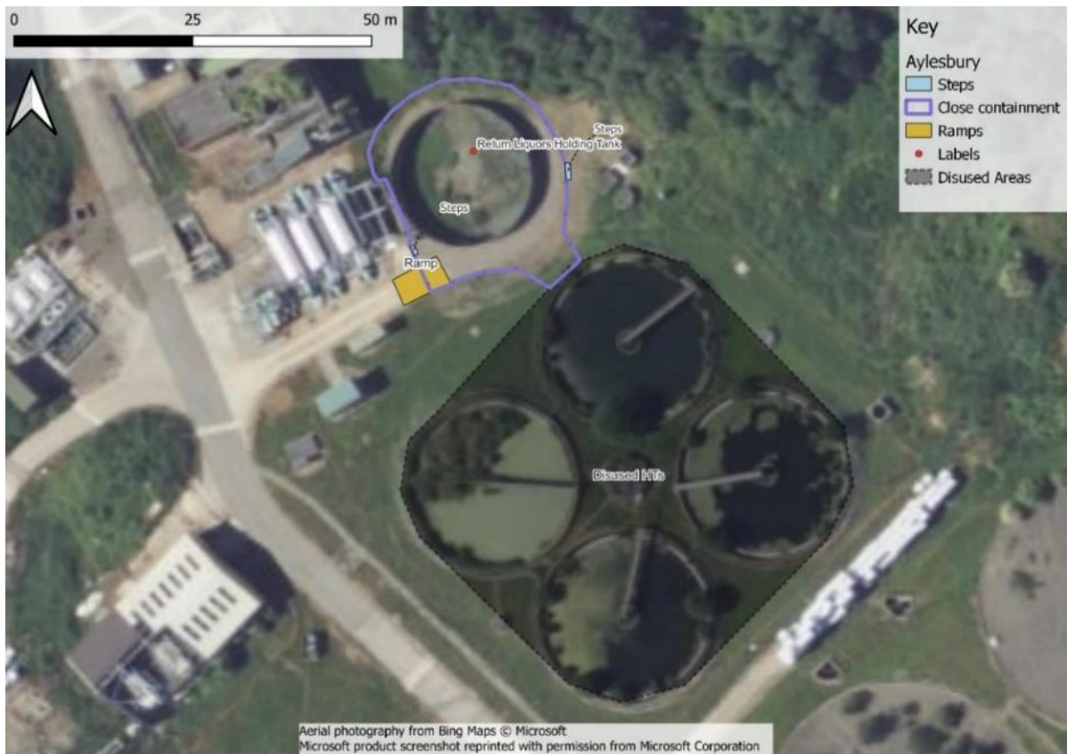
Figure 4-2 - Option 1 – Close Containment Area with a transfer channel to the disused Humus Tanks
