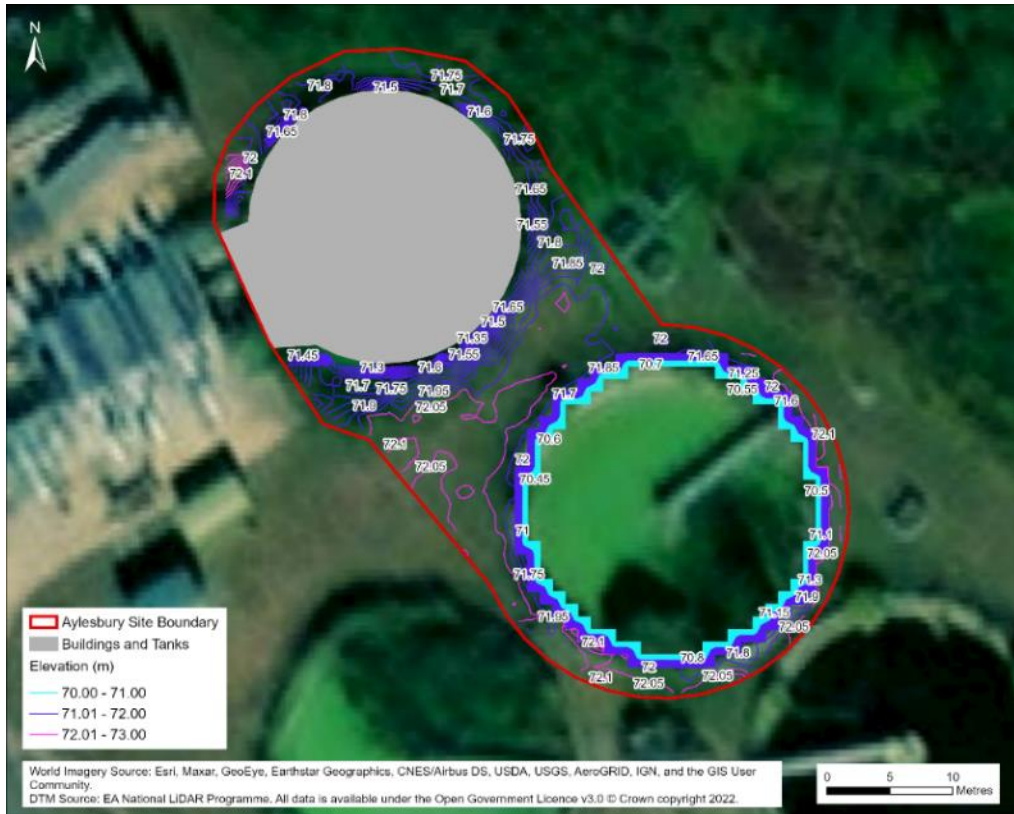
Figure 3-10 – Contour lines within containment area 3
