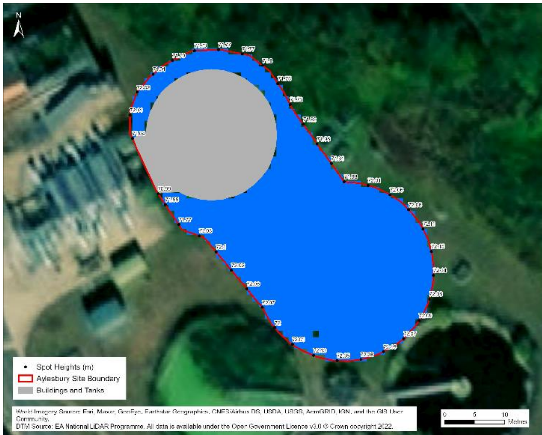
Figure 3-12 - Contained model output for area 3 showing the ground elevations at boundary
