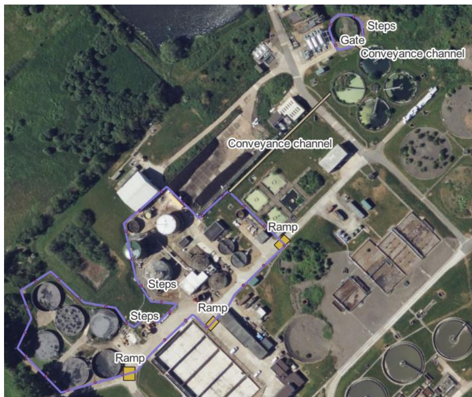
Figure 4-3 – Option 2 - 1 wide and 1 close containment area
