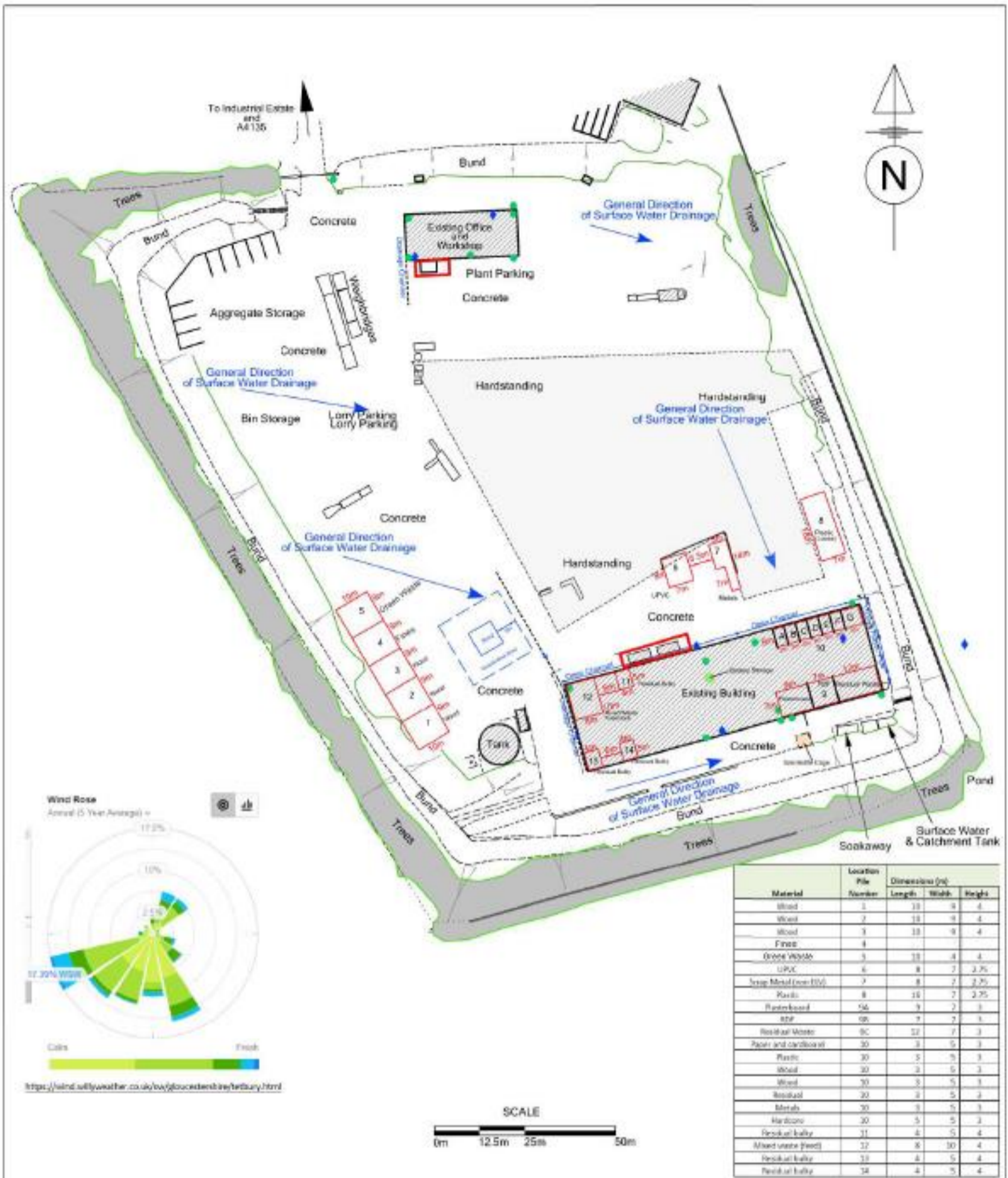
Plan showing site layout inc hardstanding where C&D waste stored and processed.
