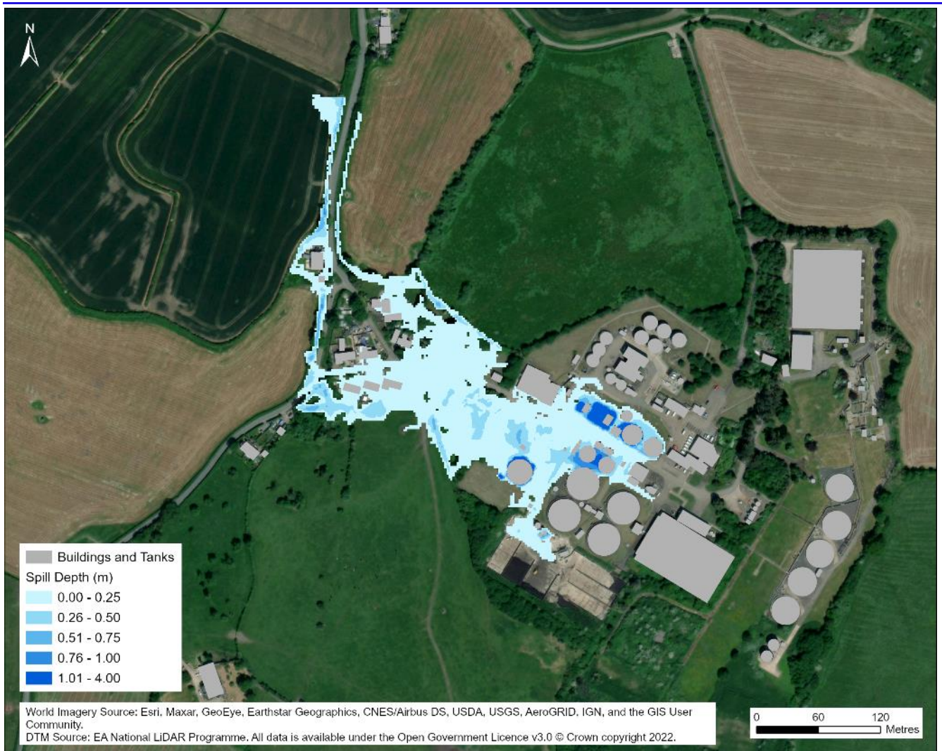
Figure 2.3 Uncontrolled spill of Hayden Sewage Treatment Works (Depth profile)
