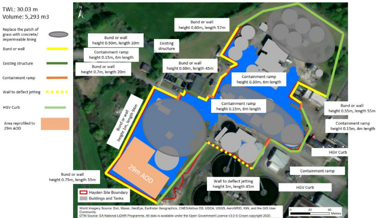
Figure 3.4 - Recommended site modifications to provide remote secondary containment for the PKTs and Digester Area
