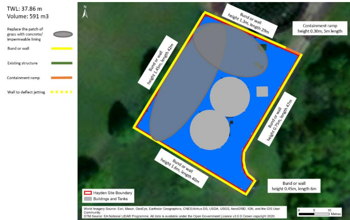
Figure 3.5 Recommended site modifications to provide remote secondary containment for Centrate Balancing Tanks Area
