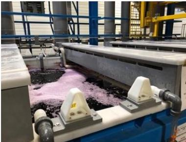
Where required the tanks are equipped with suitable hoods (placed on the tank's rim) to collect all the fumes generated during the process. Drip covers (over the hoods / between the tanks) are removable for easy inspection and cleaning.
