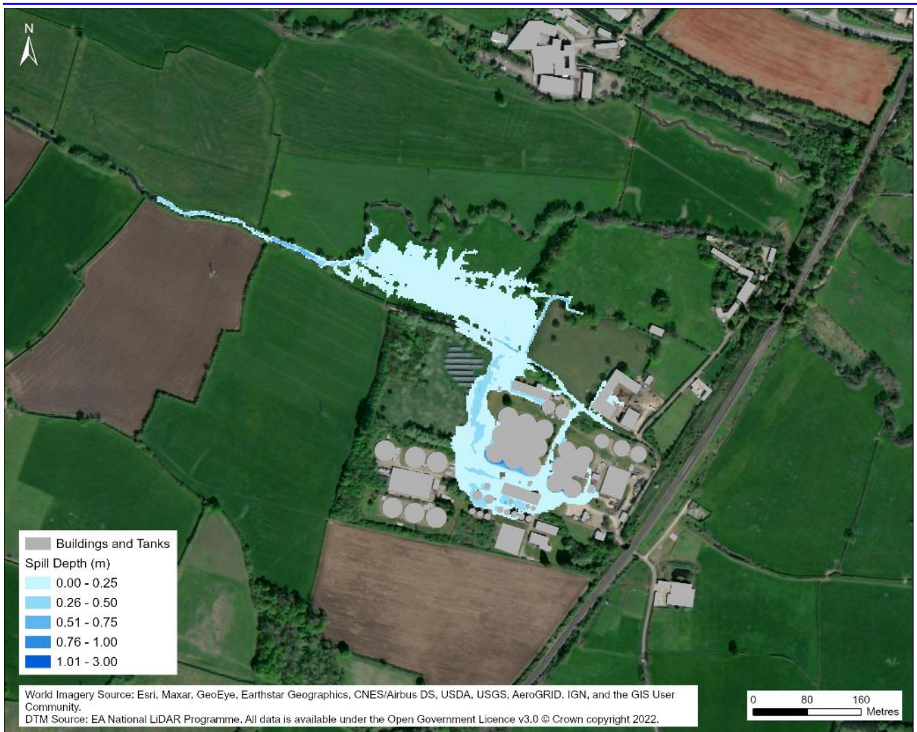
Figure 2.3 Uncontrolled spill of Stanley Downton Sewage Treatment Works (Depth Profile)
