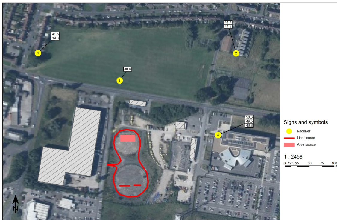
Figure 15 – SoundPlan model - sound propagation to noise sensitive properties – Tables give sound pressure level for the indicated floor heights
