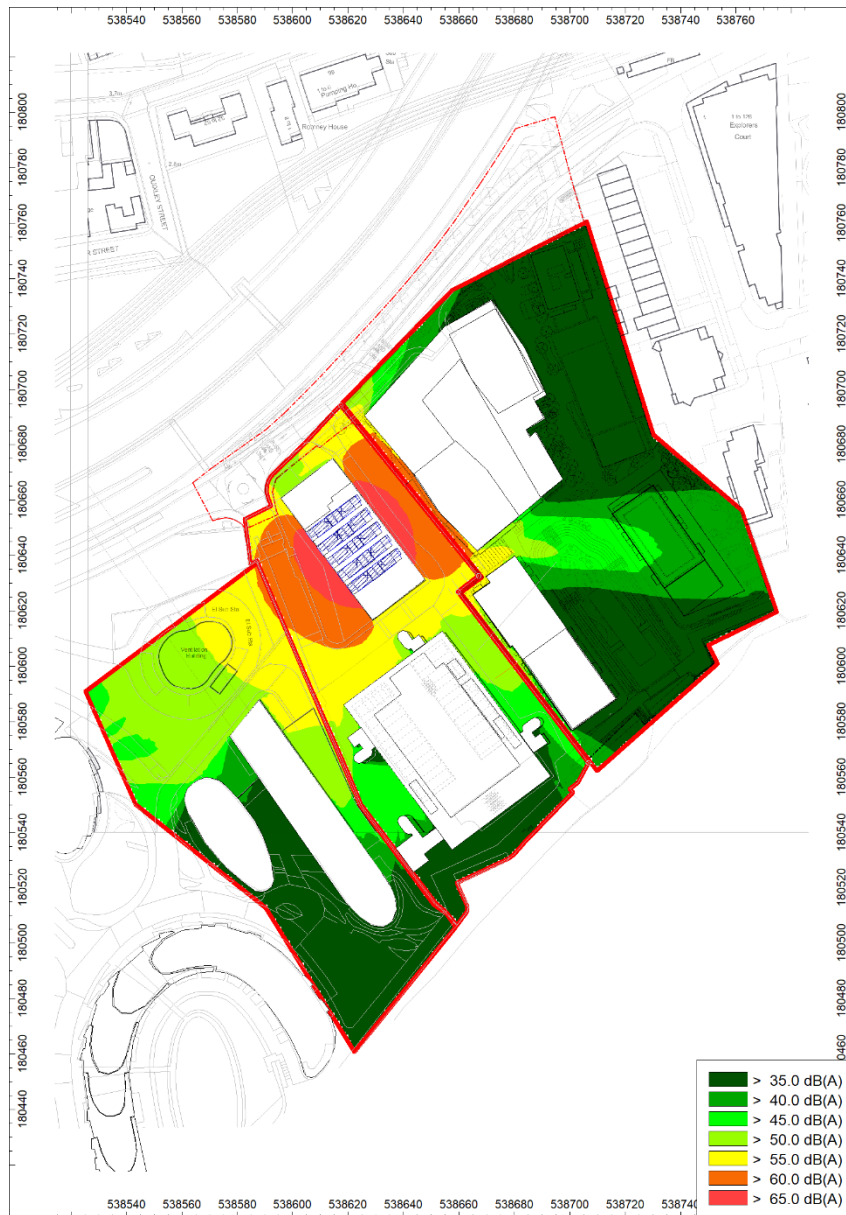
Figure 15: Noise Map at 21 metres – SSB Power Generation Plant
