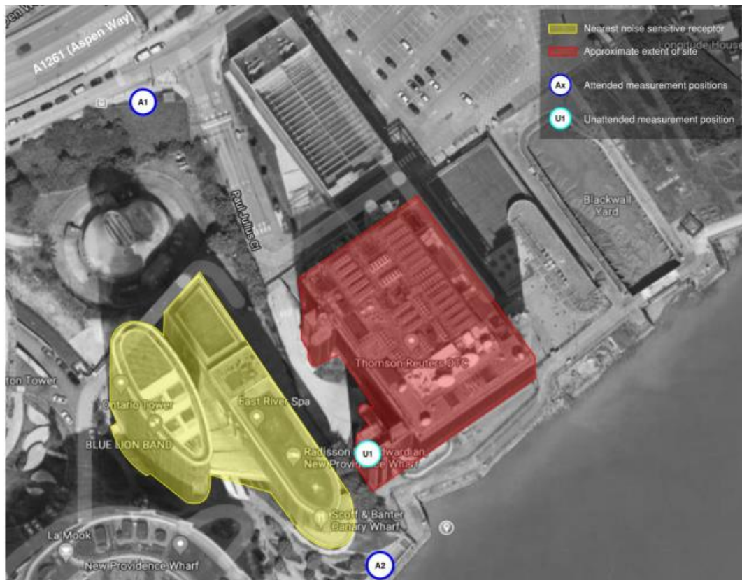
Figure 8: Sound Monitoring Positions U1, A1 and A2 – Cundall Survey – Extracted from Cundall Report
