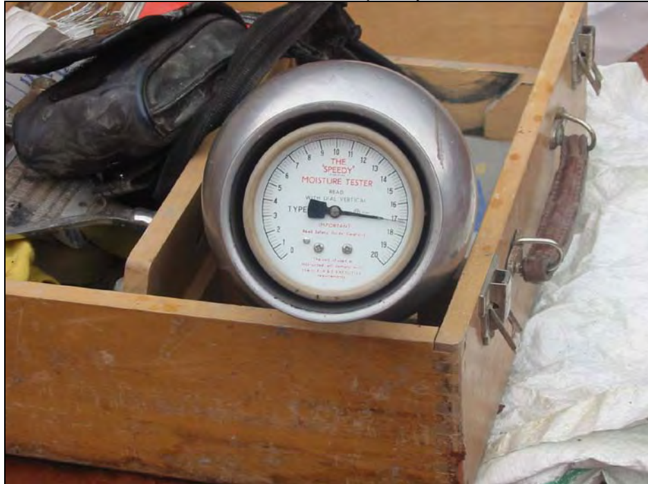
Plate 1:17% moisture on Ashworth Speedy Moisture Tester
