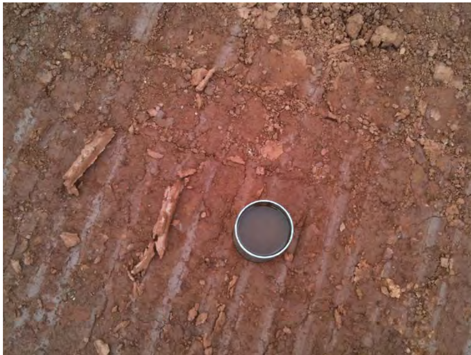
Phase 3 Section 1: Falling Head Permeability 23/03/2011
