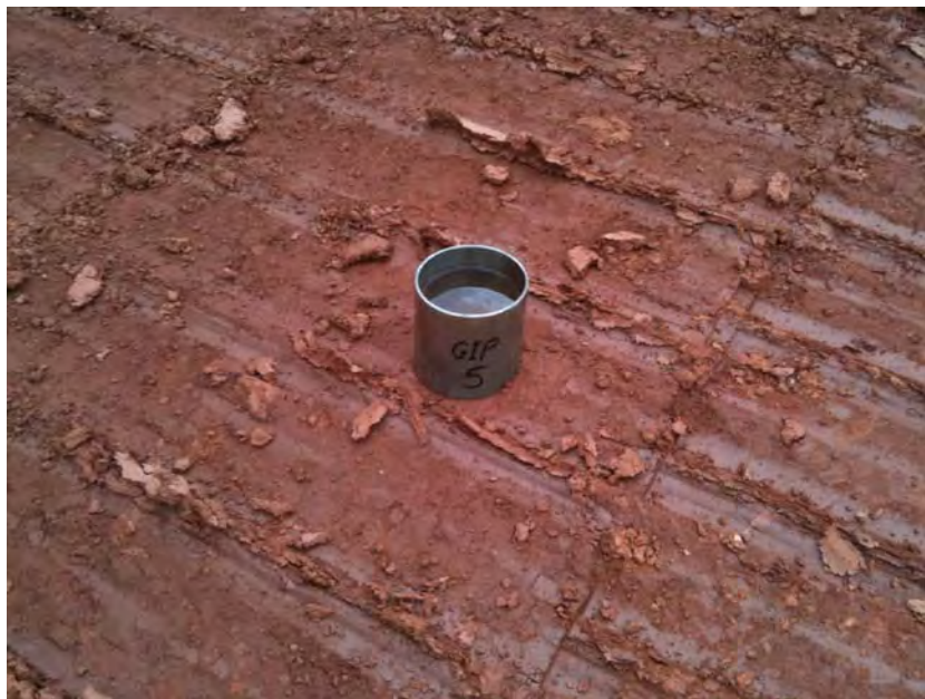
Permeability Test Phase 3 Section 2 6 th May 2011
