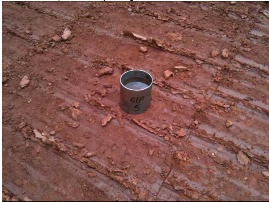
Plate 2: Core permeability falling head test on Phase 3
