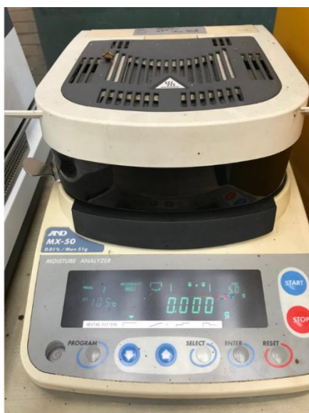
Figure 1: Typical dry Solids Analysis Machine (models may vary from site to site)
