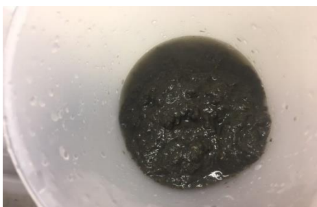
Figure 5: 6-8 DS% sewage sludge is thick but still pourable
