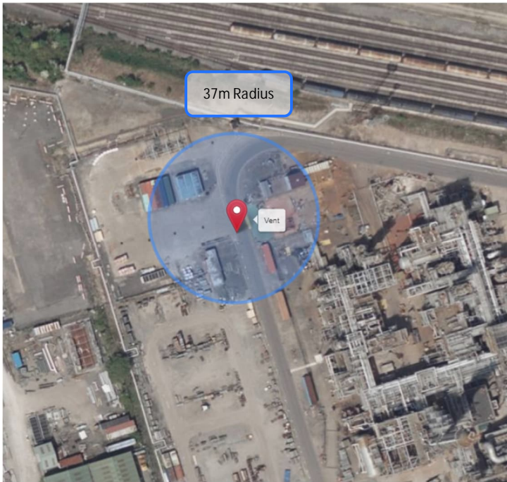
Figure 6-3 Case HP03 5,000ppm CO 2 extent at 40m elevation
