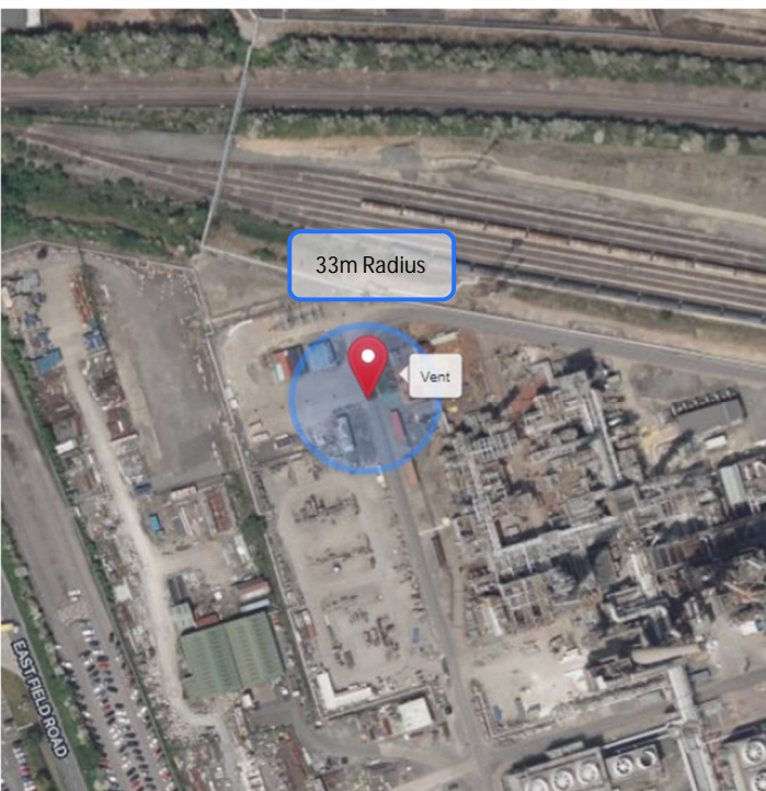
Figure 6-2 Case HP02 5,000ppm CO 2 extent at 40m elevation
