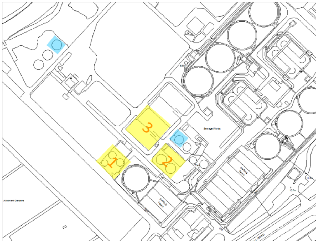
Figure 20. Sandall single tank and multi-tank installation areas.
