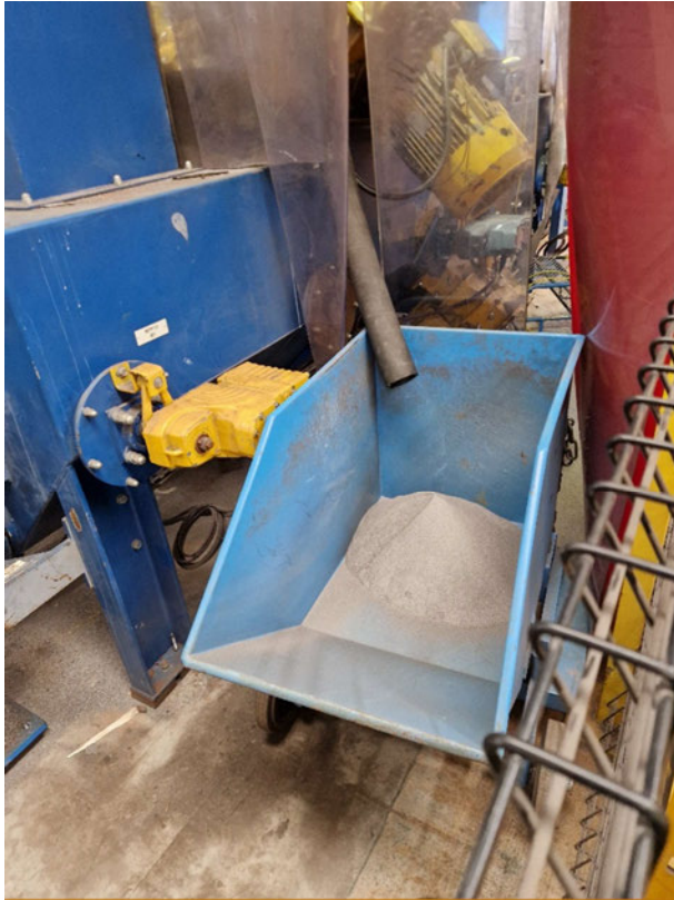
Figure 5: Spent steel shot from grit blasting
