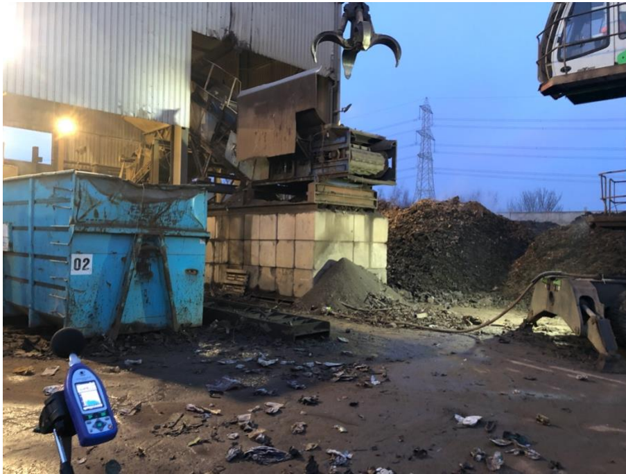
Figure E 2: Image shows the proximity of the telehandler to the shredder and its conveyor belt.
