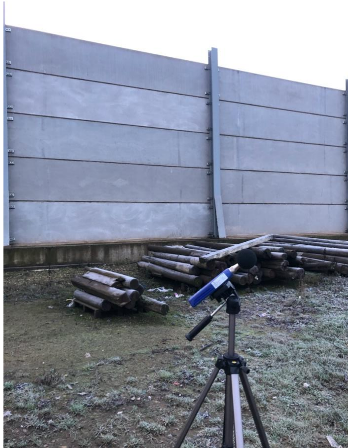
Figure E 6: Noise level meter positioned close to the boundary wall.
