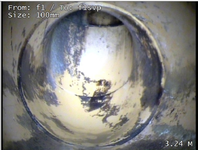
Finish node type, major connection without manhole, reference f1svp
