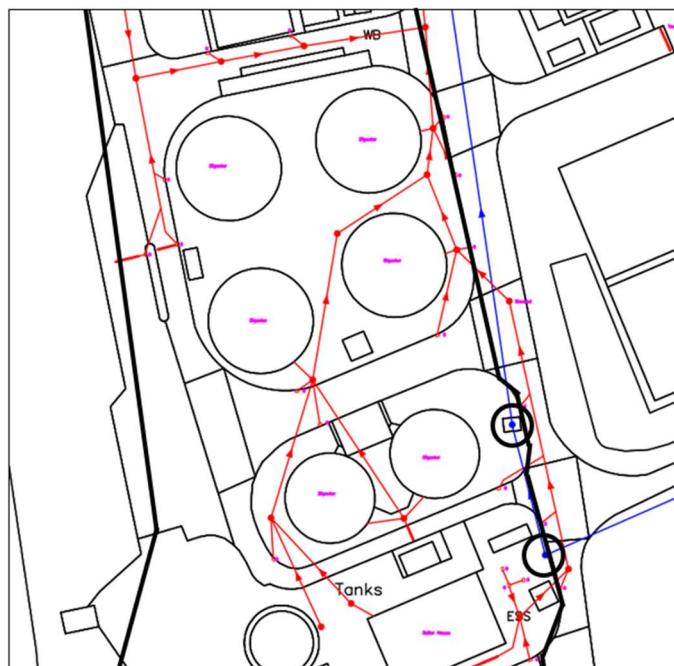
Figure 4.4 - Containment area surface water manholes to be isolated
