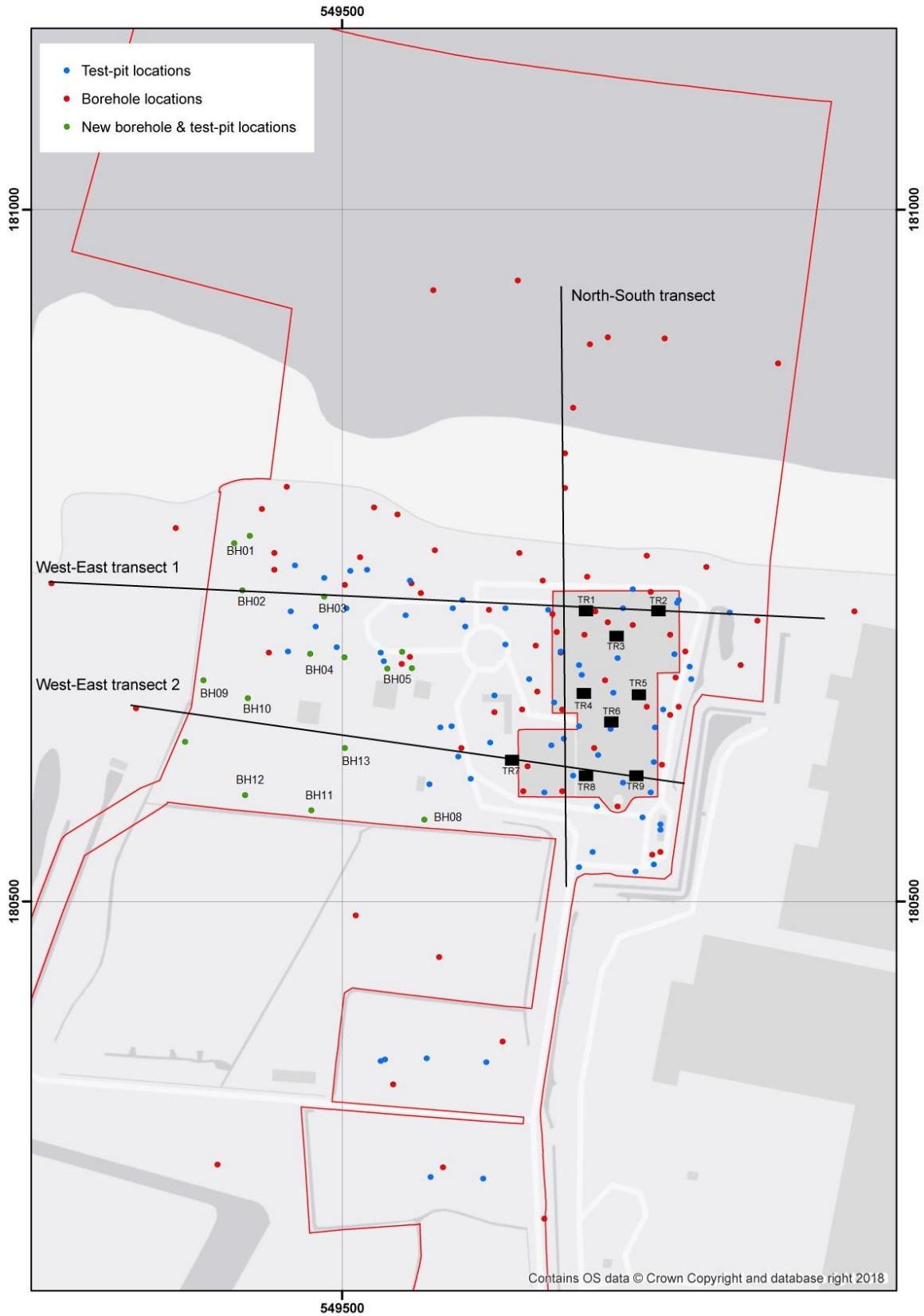
Figure 2: Proposed Geotechnical borehole locations
