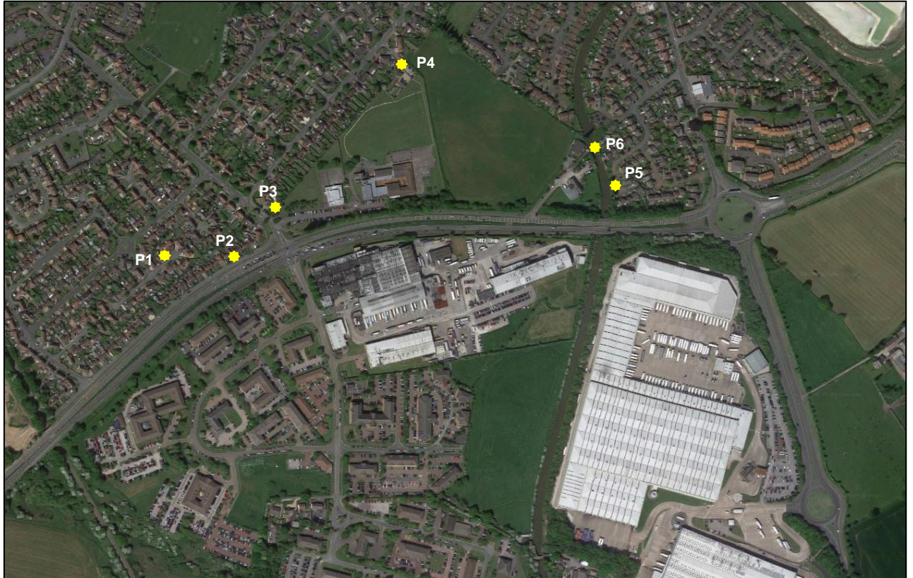
Figure 5.1: Background sound level survey measurement locations
