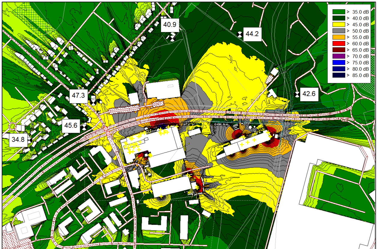
Figure 7.1: Predicted daytime noise propagation (1.5m height) – L_{Aeq}
