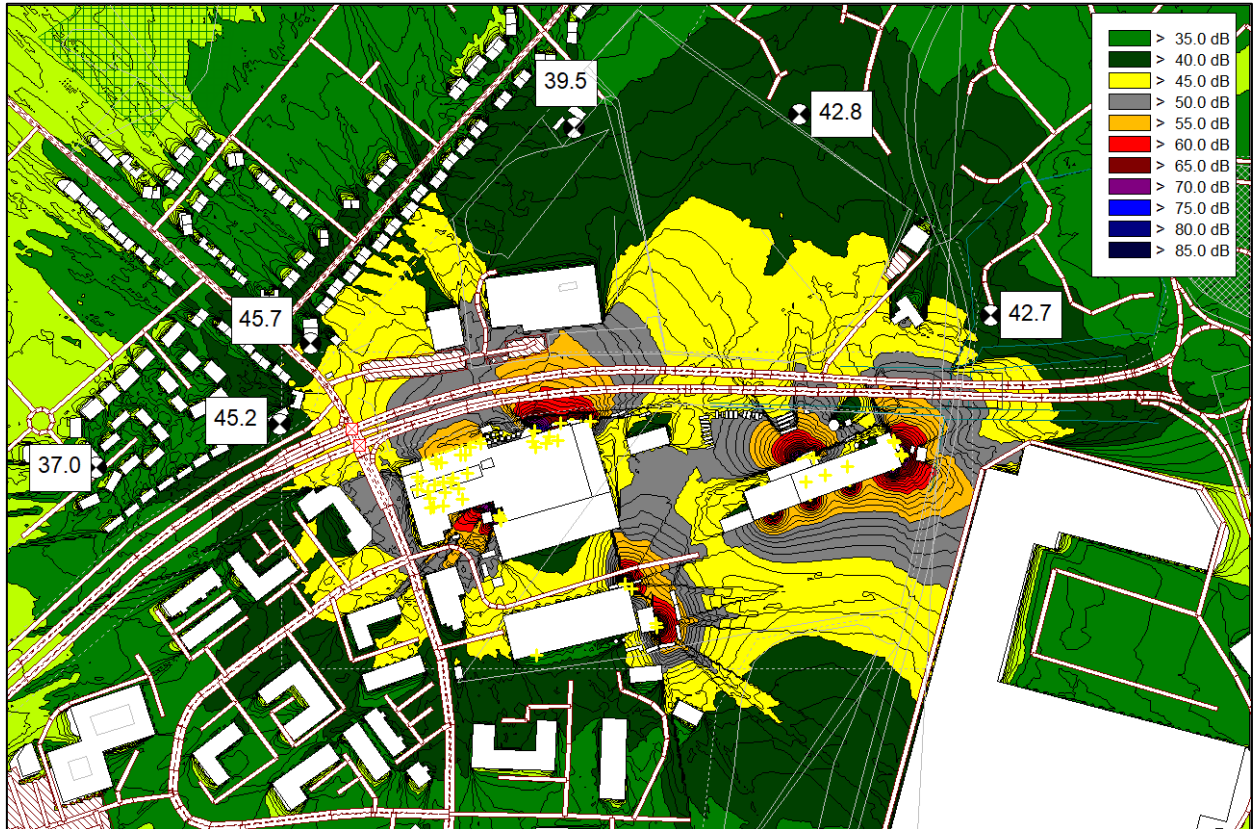
Figure 7.2: Predicted night-time noise propagation (4m height) – L_{Aeq}
