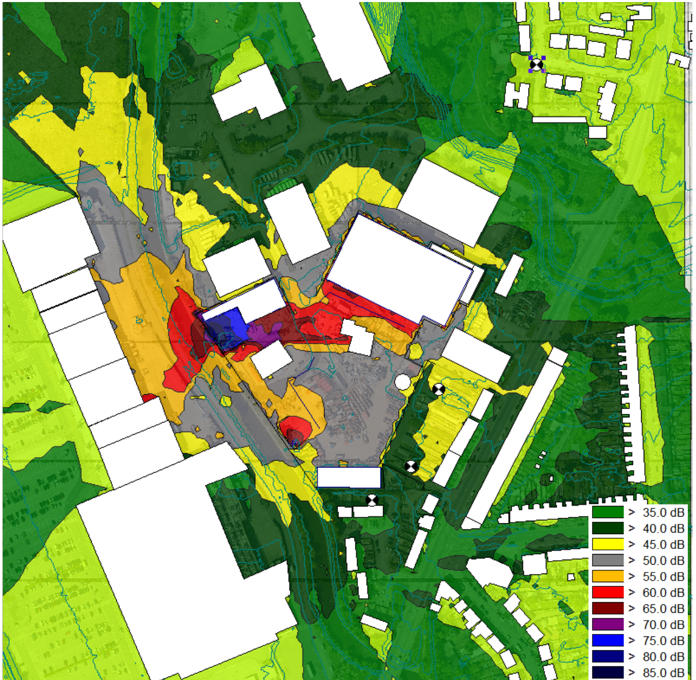
Figure 5.5 – Calculated noise levels (LAeq) associated with the typical existing operations of the site
