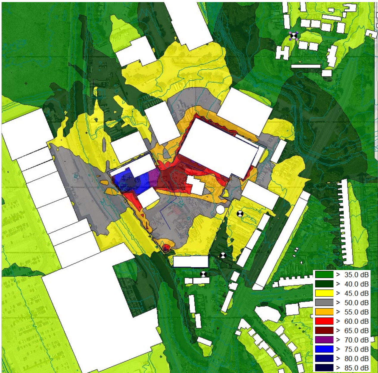
Figure 5.6 – Calculated noise levels (LAeq) associated with the site and closest noise sensitive receptors for the proposed layout.
