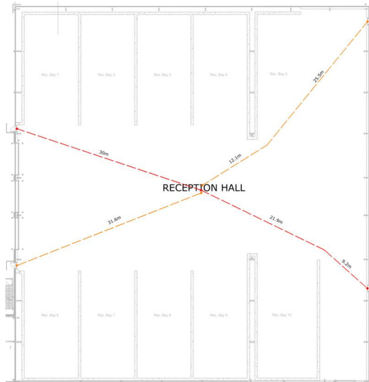
Diagram 03: Travel Distances and Escape Routes in the Process Hall
