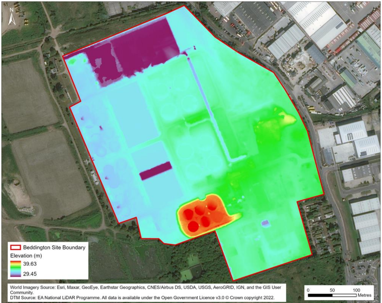
Figure 3-4 Digital Terrain Model of Beddington Sewage Treatment Works
