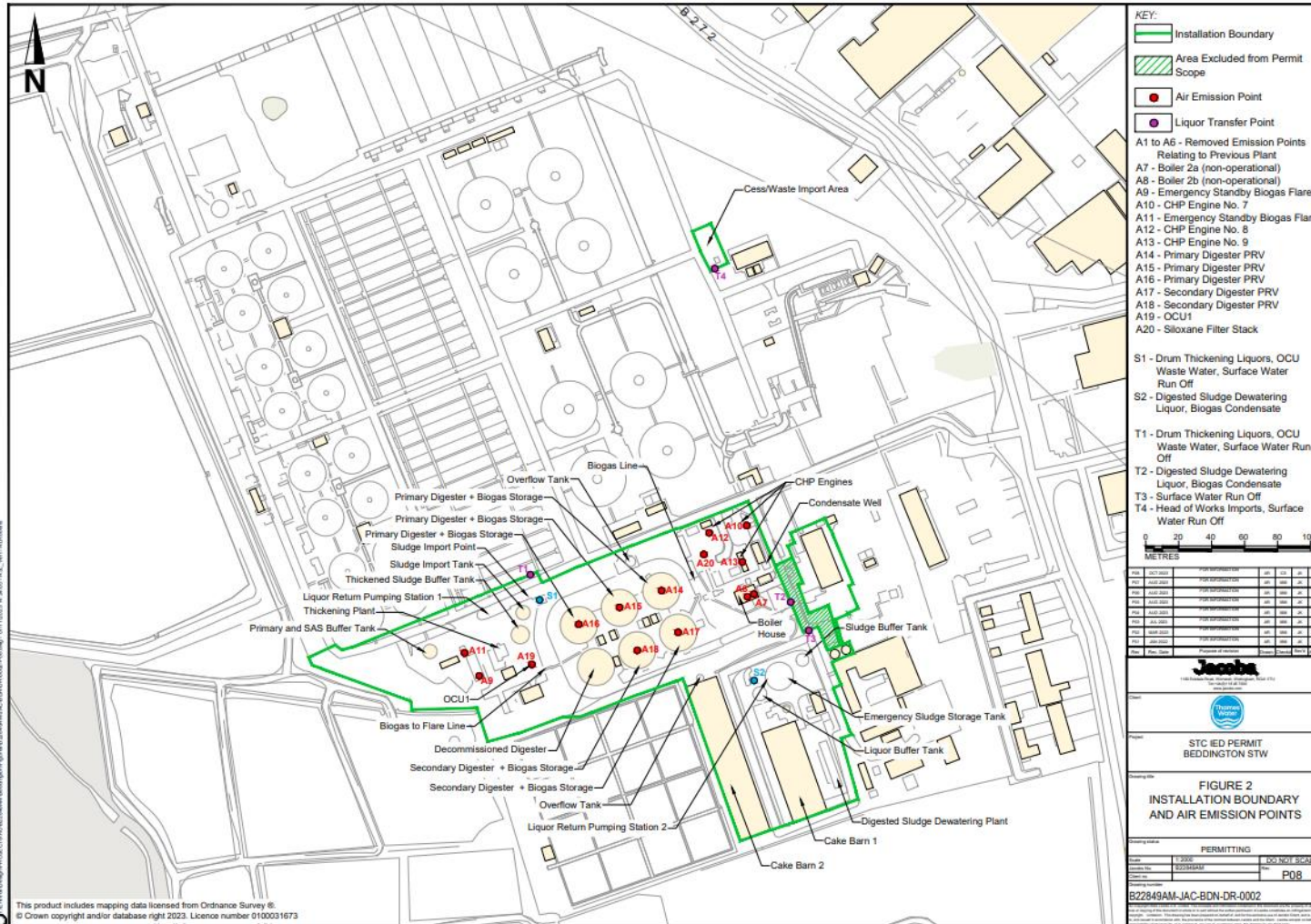
Figure C - Area Permitted under Sludge Treatment Centre Permit
