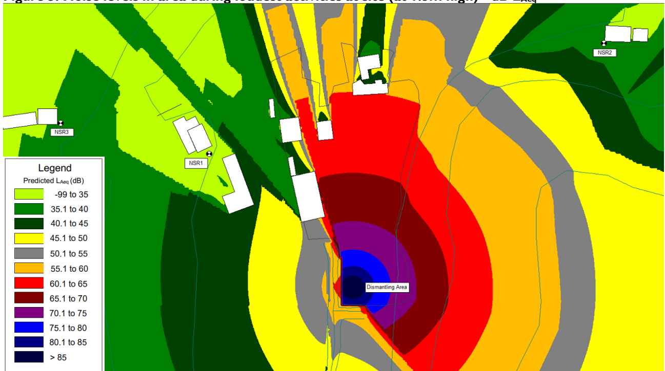
Figure 3: Noise levels in area during loudest activities at site (at 1.5m high) - dB L_{Aeq}
