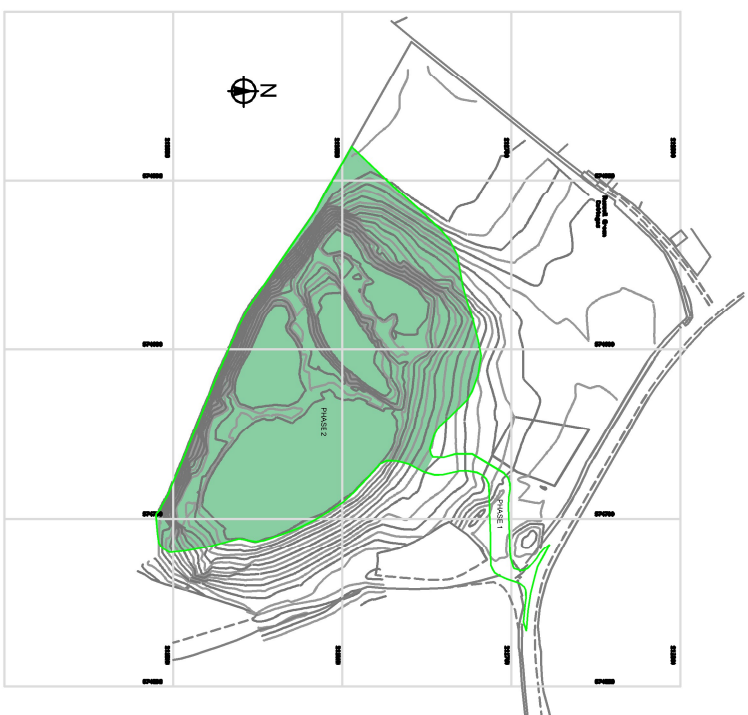
Phase 2 Removal of vegetation within working area (not between March and August). Strip topsoils, stockpile as bunding, seed.
