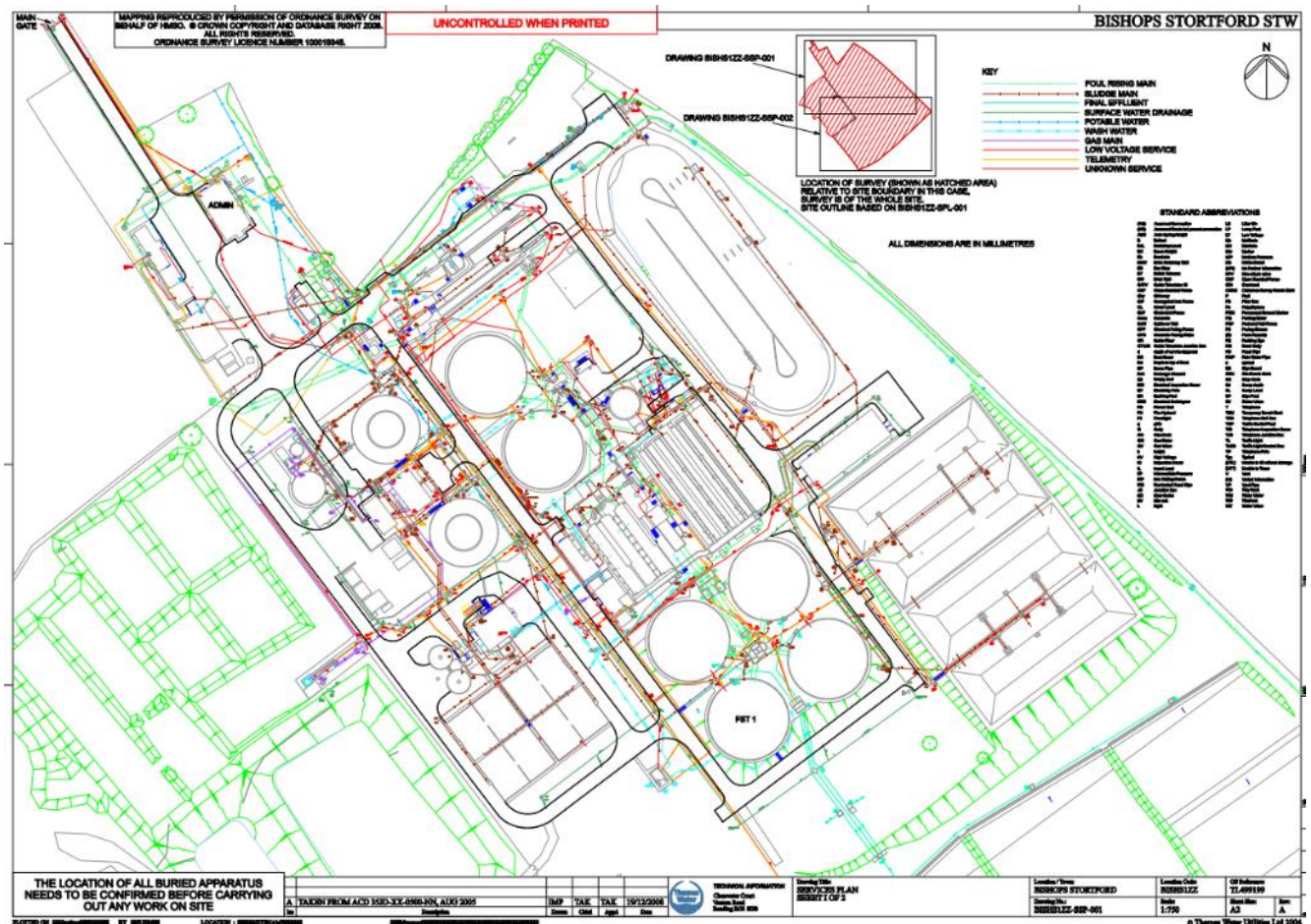
Figure 5.2 Services Plan Covering Bishops Stortford Containment Area
