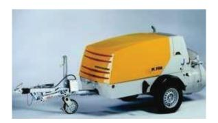
Trailer Mounted Air compressor Either delivered with other plant on the RoRo flatbed or towed using a 4wd truck such as a Land Rover
