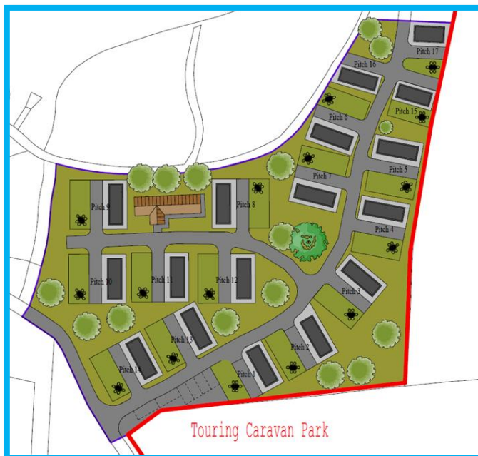
Fig 7 Indicative plan of the Touring Caravan Park. The drives will be formed in permeable gravel and where not, grass the pitches will be formed in permeable gravel or permeable construction.
