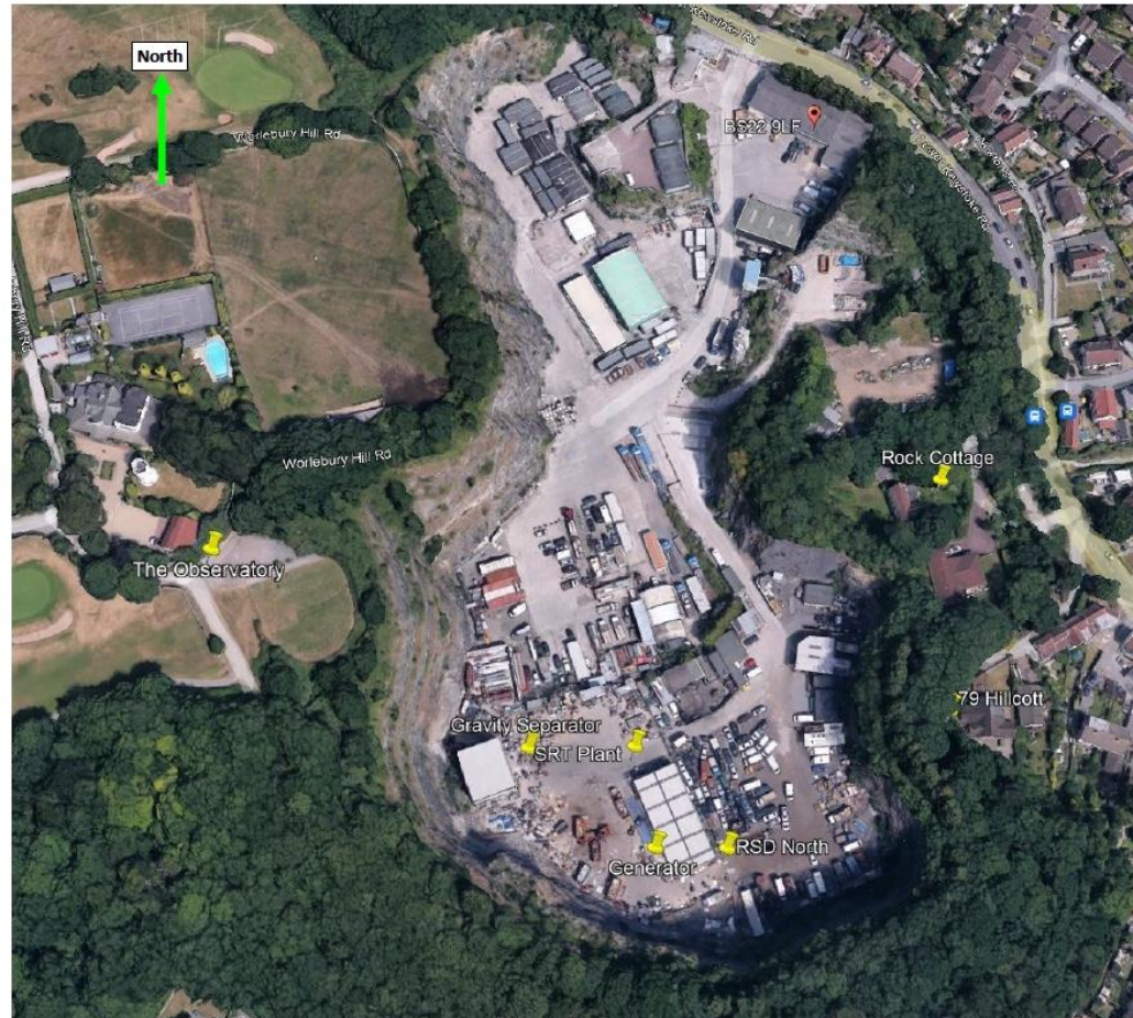
Figure 4.1 – plan showing locations of sound level measurement positions used to monitor sound from the site.
