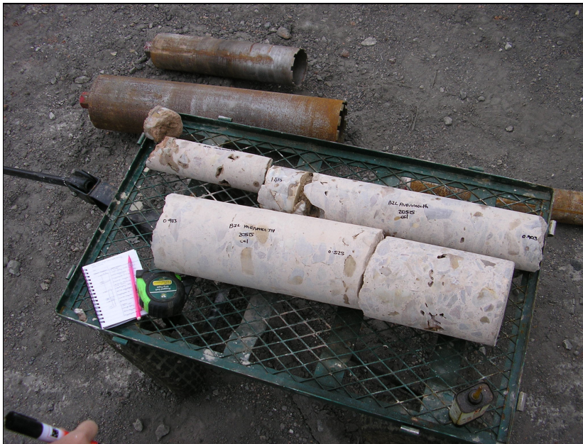
Plate 4 – Concrete cores recovered
