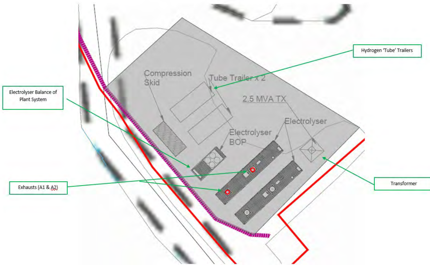
Figure 1.3: Hydrogen Plant Site Layout
