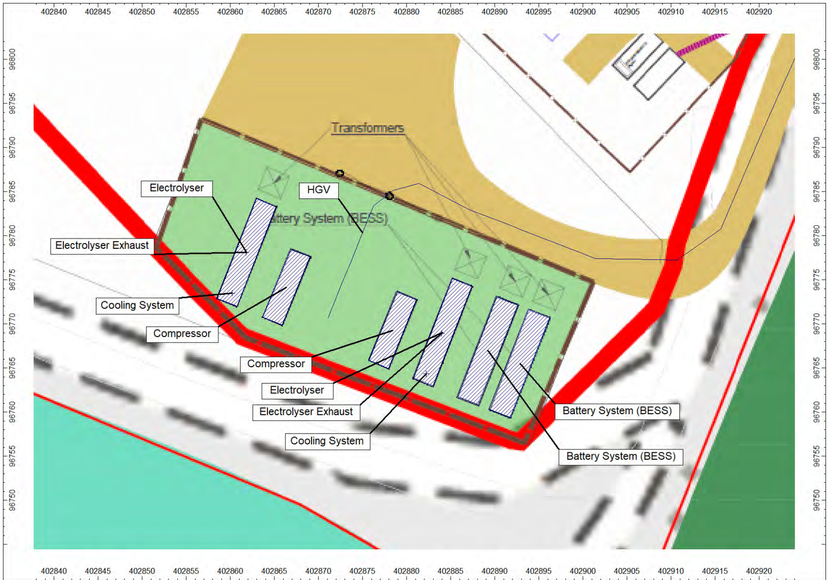
Figure C1: Site plan indicating grid coordinate references x, y coordinates for all external modelled noise sources
