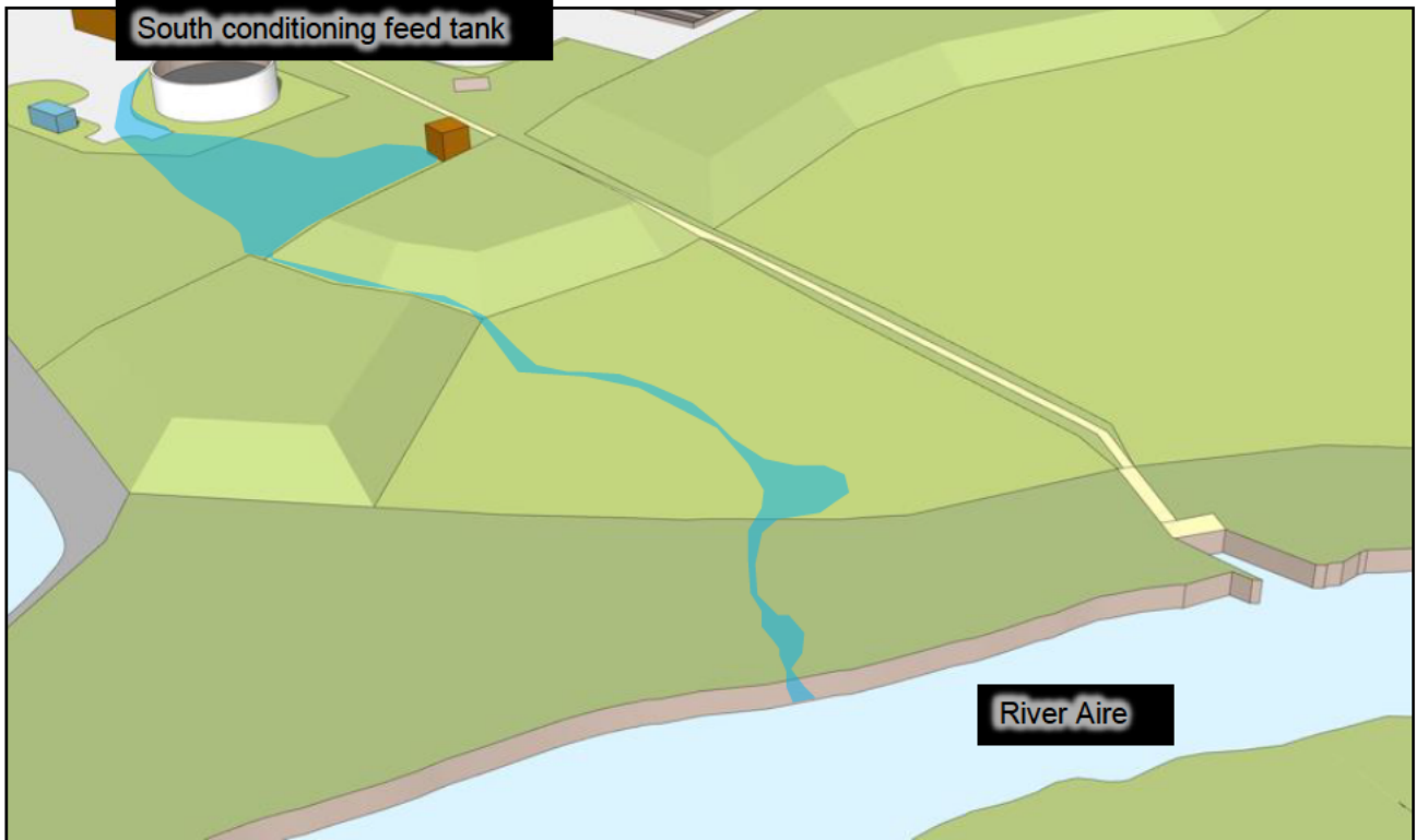
Figure 32. Direct spill pathway to River Aire via the south conditioning feed tank in the DW area (east).
