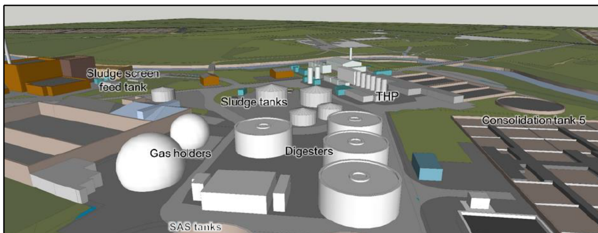
Figure 7. Tanks within the AD area.
