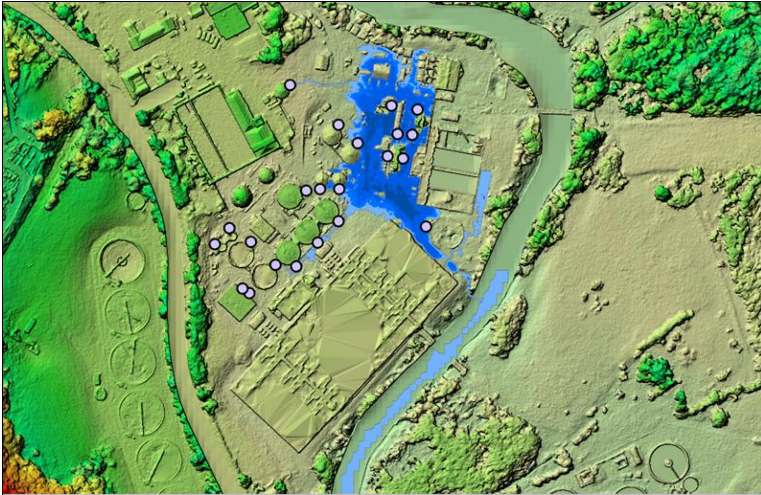
Figure 26. AD area: model showing unmitigated result of spills from existing tanks.
