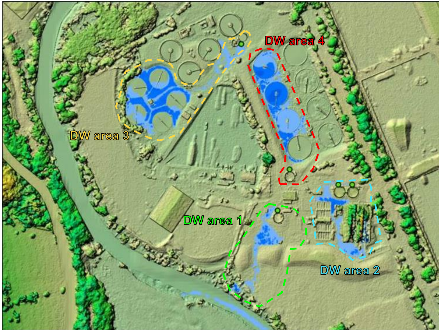
Figure 27. DW area: model showing unmitigated result of spills from existing tanks in DW area's 1 to 4.
